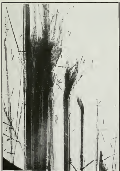
Break in asbestos fibre from West Griqualand, South Africa. Magnified 350 diameters.
